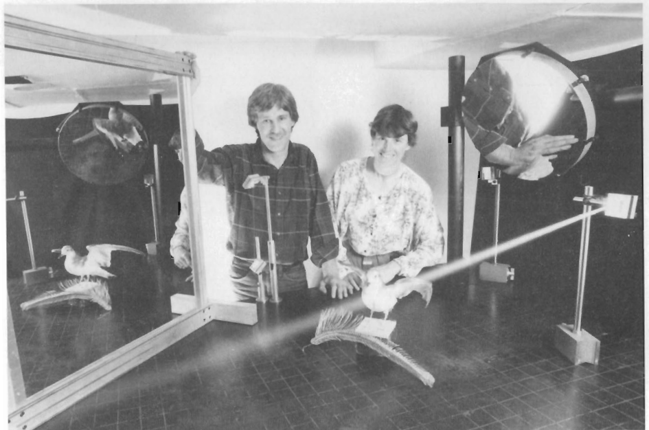
A vibration-absorbing, two-ton 'pingpong table,' a series of mirrors and a laser beam help Microwave Technology Division's Greg Cherry and his wife create holograms.
